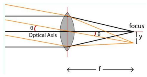
The term is often used in photography, where it refers to the "speed" of the camera. The larger the focal ratio, the "slower" the camera, as the amount of light falling on a given area of the focal plane is smaller. For larger f at fixed D, the plate scale ps is smaller and hence the light is spread out over a larger area. For a "faster" camera, the reverse is true.
