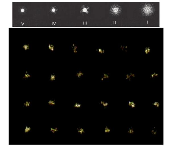
Ground-based telescope resolution is determined by the atmosphere, rather than aperture size. The central maxima of a Point Spread Function (PSF) expanded by turbulence is called *seeing disc*, and its FWHM is *seeing*.
