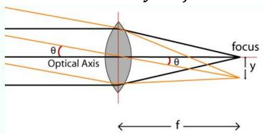
If an astronomer wishes to study an object of angular size in high spatial detail, ps needs to be small, and therefore a long focal-length telescope is required.
