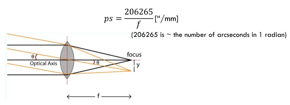
For direct imaging, the angle on the sky subtended by the detector pixel is  $\theta=ps\ d_{pix}$ , where  $d_{pix}$  is the physical pixel size in mm.
