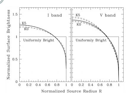
Thick lines show how much fainter the K giant becomes at its edges in the red I (left) and blue-green V filter (right). If the star emitted a uniform amount of light across its whole stellar disk, the profile would look like the straight solid black line instead
