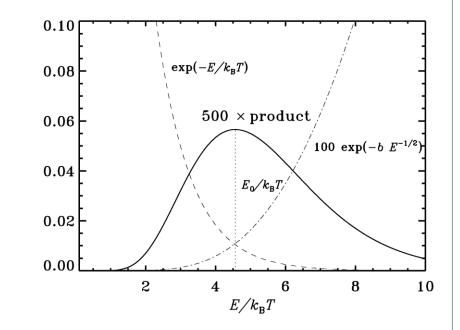
The Boltzmann probability distribution for kT = 1 keV, the Gamow factor for the case of two protons, with  $E_G = 500$  keV, and their product. Scaled up by large factors for display purposes.
