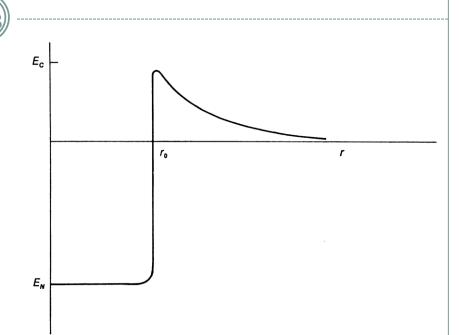
Schematic potential energy between two nuclei. For  $r < r_0$  the attractive nuclear forces dominate; for  $r > r_0$  Coulomb repulsion dominates.
